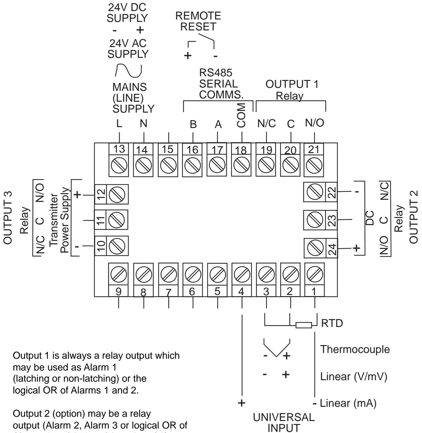
Output 1 is always a relay output which may be used as Alarm 1 (latching or non-latching) or the logical OR of Alarms 1 and 2.
