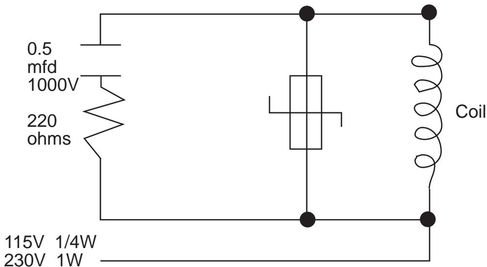
Contacts - Arcing may occur across contacts when the contact opens and closes. This results in electrical noise as well as damage to the contacts. Connecting a RC network properly sized can eliminate this arc.
